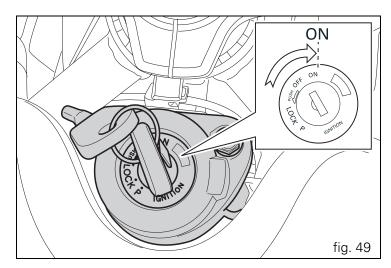
Note It is possible to start the engine with side stand down and the gearbox in neutral. When starting the bike with a gear engaged, pull the clutch lever (in this case the side stand must be up).
