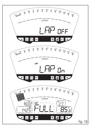
When the LAP function is set to Off in the menu, the current "lap" is not stored.
