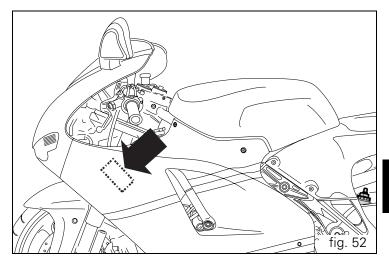
USB data logger A USB data logger (1) is supplied as a kit. To use the data logger, place it under the seat with the plug (2) installed and the main wiring harness connector (3) connected. Please refer to the "USB data logger" procedure outlined in paragraph "LCD - Parameter setting/display".
