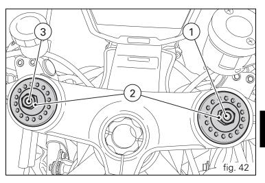
STANDARD factory setting is as follows: Compression: top adjuster (left fork leg) 10 clicks; bottom adjuster (fork bottom) 10 clicks. Rebound: 12 clicks. Spring preload (fig. 42): 3 mm (1 turn = 1 mm). Spring stiffness: 10.5 N/mm.
