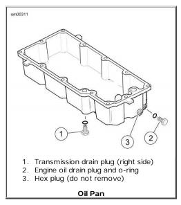
4. Inspect the oil drain plug o-ring for cuts, tears or signs of deterioration. Replace as necessary.
