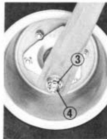
③ Axle Nut ④ Cotter Pin
