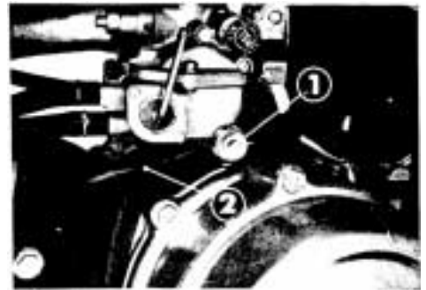
① Drain screw knob ② Drain tube
