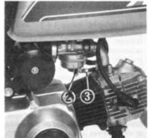
② Drain screw ③ Drain tube
