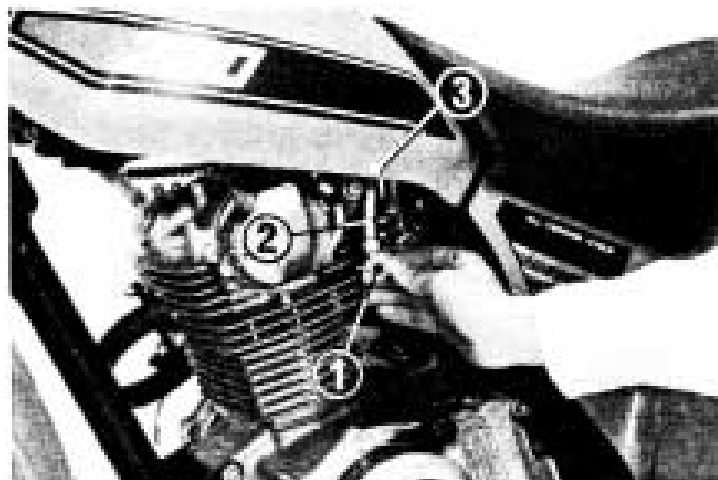
(1) Fuel valve (2) Fuel filter
