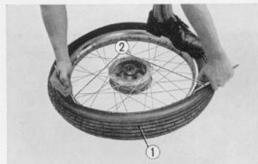
Fig. 4.87 Removing tire ① Tire ② Tire lever
