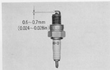
Fig. 5.10 Measuring spark gap
