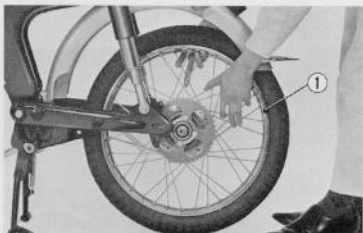
Fig. 4.73 Removing rear wheel ① Rear wheel
