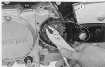
Fig. 4.94 Disconnecting drive chain ① Drive chain
