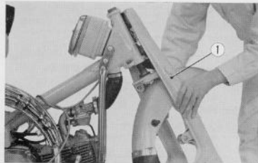
Fig. 4.36 Removing front fork ① Front fork
