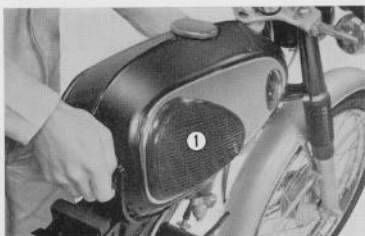
Fig. 4.42 Removing fuel tank ① Fuel tank
