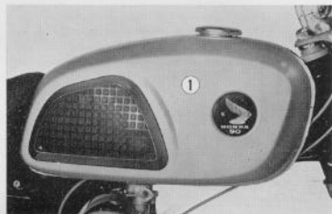
Fig. 4.39 B Fuel tank (CL 90) ① Fuel tank
