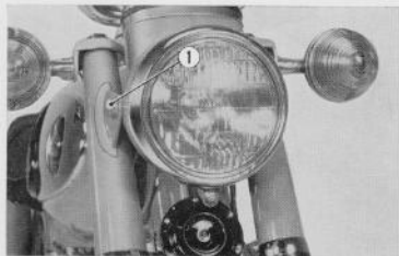
Fig. 4.25 Removing headlight ① 8×22 hex bolt
