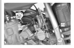
(1) connecting and insulator tube clamp screws(2) float bowl plug
