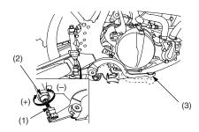
(1) lock nut (2) adjusting bolt (3) rear brake pedal (+) raise the pedal height (-) lower the pedal height
