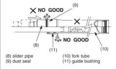
Record the rebound damping adjuster position and turn the adjuster screw (12) counterclockwise until it stops. 10.Hold the fork tube (10), then remove the fork cap (2), from the fork tube. Gently slide the fork tube down onto the lower end of the slider pipe (13).
