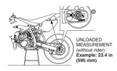
3. Measure the loaded with rider dimension. Remove the workstand. With two helpers available, sit as far forward as possible on your CR's seat, wearing your riding apparel. Ask one helper to steady your CR perfectly upright so you can put both feet on the pegs. Bounce your weight on the seat a couple of times to help the suspension overcome any situation and settle to a good reference point.
