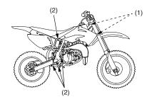
(1) steering head bearings(2) suspension pivot points
