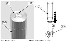
(2) fork cap (10) fork tube (12) adjuster screw(13) slider pipe, lower end
