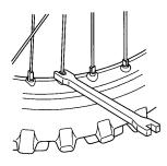
Clean the sides of the drive chain with a stiff, nylon parts-cleaning brush. Lubricate and adjust the chain as necessary.
