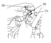
(1) piston pin (2) "IN" mark (3) piston pin clip
