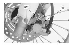
(6) caliper (25) caliper mounting bolts
