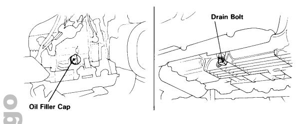
2. Remove the under cover and oil filter with a filter wrench. Discard the oil filter.
