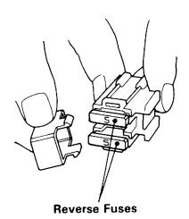
When frequent fuse failure occurs, it usually indicates a short circuit or an overload in the electrical system. See your authorized Honda dealer for repair.
