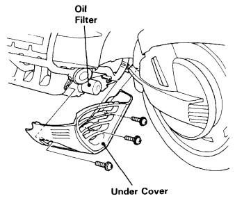
3. Apply a thin coat of engine oil to the new oil filter rubber seal.
