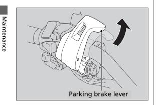
Place your motorcycle on a firm, level surface. Stop the engine and push your motorcycle while applying the parking brake lever to check the efficacy of the parking brake.
