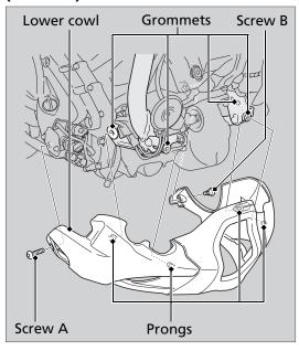
The lower cowl must be removed to service the coolant reserve tank, to replace the engine oil filter and clutch oil filter.
