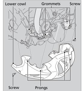
The lower cowl must be removed to service the coolant reserve tank, to replace the engine oil filter.
