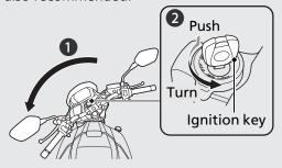
ON Turns electrical system on for starting/riding.
