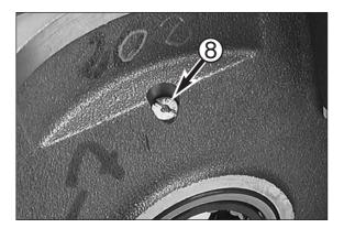
The oil pump casing <sup>(C)</sup> must not have any score marks or seizing marks.
