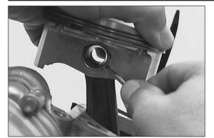
Remove the wire circlip and the push piston bolt from the piston. \_ Dismount the piston.
