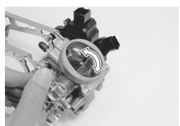
Apply thin coat of the engine oil to the new cushion seal 3, and the O-ring 4.
