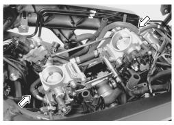
• Loosen the throttle body clamp screws.
