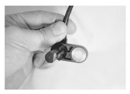
• Check that no wheel speed sensor rotor teeth are broken and that no foreign objects are caught in the wheel speed sensor.
