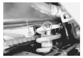
• Remove the battery case bolts.
