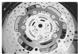
• Remove the front wheel speed sensor rotor 3.
