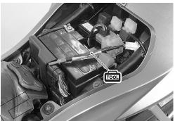
While the DTCs are being output, set the special tool to OFF
