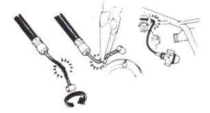
Rubber parts may become deteriorated when old, and prone to be damaged by solvent and oil. Check these parts before installation to make sure that they are in good condition, replace if necessary.
