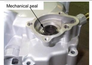
Turn pump rotor clockwise and remove.
