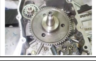
Remove mounting plate, starter reduction gear, and the shaft.
