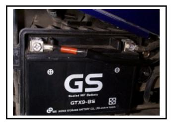
Disconnect the cable positive terminal from the relay.
