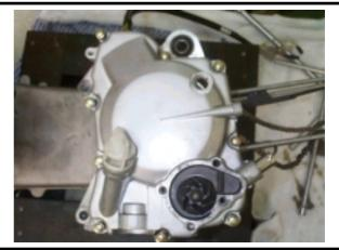
Install the dowel pin and new gasket. Install the water pump cover with three bolts.
