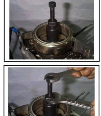
Pull out flywheel with A.C.G. flywheel puller. **Tool: A.C.G. Flywheel puller**
