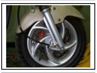
Tighten the nut for the wheel axle. **Torque value: 10.0 ~ 12.0 kgf-m**
