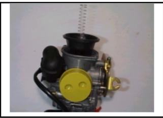
Install vacuum piston to carburetor body and align the indent on the diaphragm.
