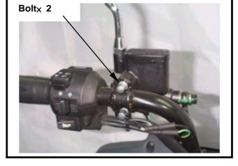
Loosen the lock bolt for the handle fix bolts. (Bolt  $\times$ 4)
