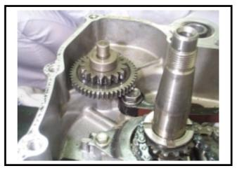
Install starting clutch gear onto crankshaft.
