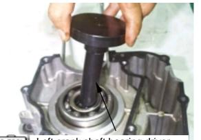
Left crank shaft bearing driver
