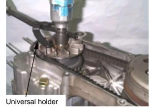
Install the clutch with universal holder, and then tighten nut to specified torque value. **Torque value: 5.0~6.0 kgf-m**
