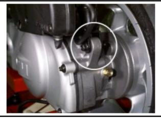
Remove the lower mounting bolt of left shock
