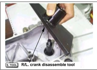
Refer to chapter 18: Special tools Special tool : R/L. crank case disassemble/install tool SYM-1120000-H9A
