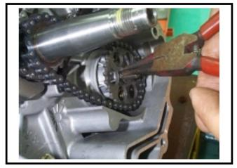
Install starting gear and generator.
