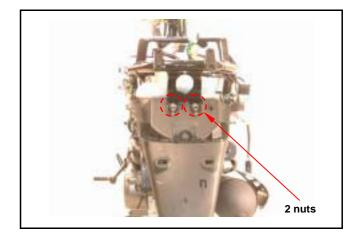
• Remove 1 bolt from front rear fender then remove the rear fender.
