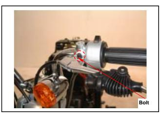
Remove front and rear brake lever bracket mounting bolt.
