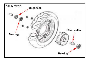
Remove dust seal, bearing and side collar.
