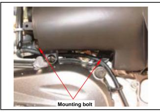
Support the engine and then remove shock absorber lower mounting bolt.
