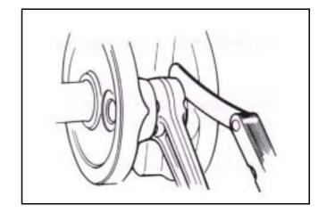
Measure the radial clearance of connecting rod big end at X-Y directions as diagram show.
