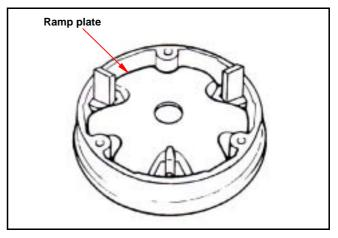
Apply with grease 4~5g to inside of movable drive face, and install drive face boss.
