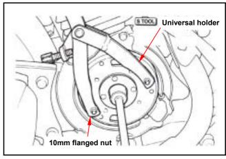
Remove the flywheel with rotor puller.
