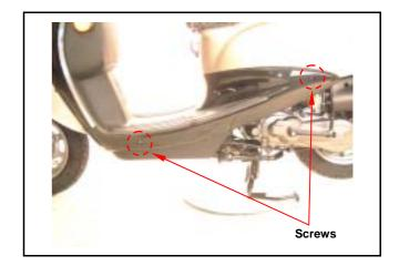
Slide the side cover backward so that and remove the side cover
