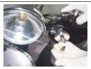
Tail light / Brake light / Rear winker light Remove 2 screws and then remove tail light lens.
