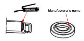
Remove residues of the old gasket or sealant before reinstallation, grind with a grindstone if the contact surface has any damage.
