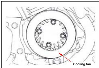
Hold flywheel with universal holder. Support the flywheel and the remove the 10 mm nut on the flywheel.
