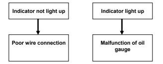
3. Disconnect oil gauge coupler, and check voltage between wire and ground.
