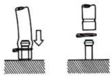
Rubber and plastic boots should be properly reinstalled to the original correct positions as designed.
