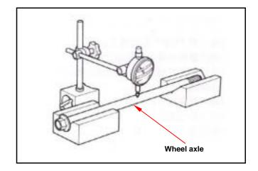
Place the wheel on to a rotation seat, and turn the wheel to check it bearing free play. If the bearing is noisy or its free play is too much, replace it.
