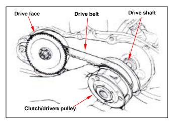
Install the clutch with universal holder, and then tighten nut to specified torque value.
