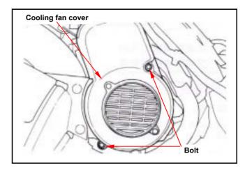
Remove four bolts, and then take out the cooling fan.
