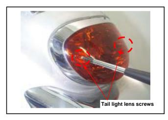
Replace tail light and brake light bulb. Install the all removed parts.
