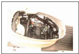
Remove 4 screws from the two side cover, and then remove the side cover.
