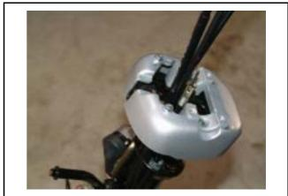
Remove the steering stem lock nut. Remove top cone race and front fork.
