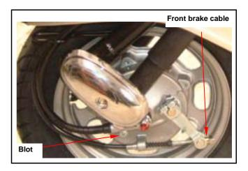
Remove front wheel axle nut, and then pull out the axle then remove the wheel.
