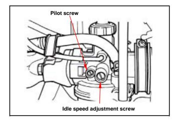
Adjust the idling after warn up engine for 10 minutes.
