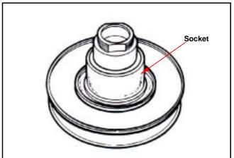
Remove guide pin, guide pin roller, and driven pulley, and then remove O-ring & oil seal seat from sliding pulley.
