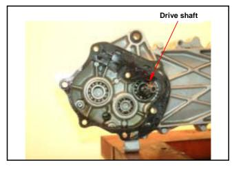
Remove drive shaft oil seal and bearing from left crankcase.
