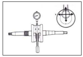
Place the crankshaft on a V-block, measure run-out points A and B of the crankshaft with dial gauge.
