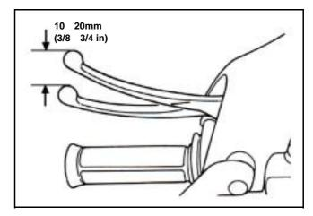
Adjust the free play by turning the front brake adjustment nut if necessary.
