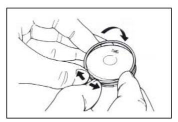
Check if cylinder and piston are worn or damaged, and then clean carbon deposit on exhaust opening area as the diagram shown.
