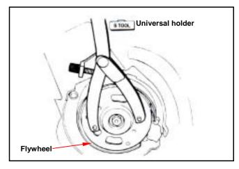
Tighten nut to specified torque.
