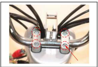
Remove handle and front brake lever bracket.
