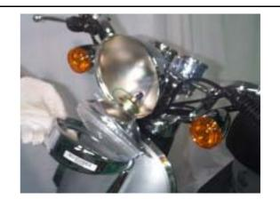
Remove bulb seat and replace the bulb. Install the all removed parts.
