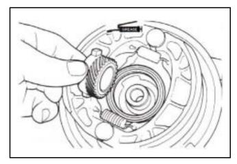
Align the flange part on the speedometer gear with the slot of wheel hub.
