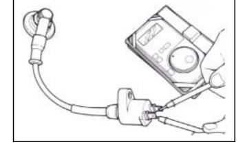
Remove the high voltage coil cap, and measure its negative (-) terminal for the secondary coil resistance.
