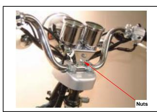
Remove bolt / nut from head light stay and then remove the head light.
