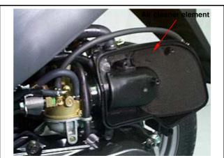
Soap the element into cleaning engine oil and element seat and then install the air cleaner cover.
