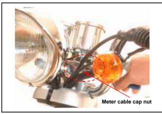
Remove 2 cap nuts from meter ASS'Y and then remove meter ASS'Y.
