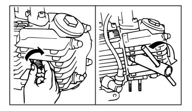
Before installing the spark plug, measure the electrode gap with a wire thickness gauge; adjust the gap to specification as necessary.
