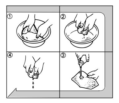
Apply recommended oil to the entire surface of the filter and squeeze out the excess oil. The element should be wet but not dripping.
