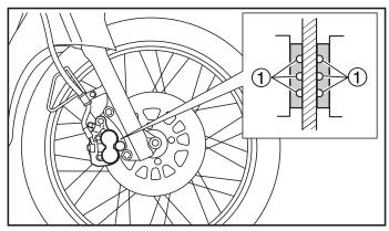
1. Brake pad wear indicator groove (×3)
