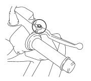
The pivoting point of the brake lever must be lubricated at the intervals specified in the periodic maintenance and lubrication chart.
