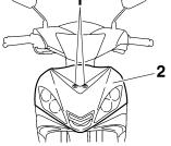
1. Screw and license bracket plate 2. Cowling A
