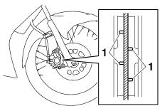
1. Brake pad wear indicator groove
