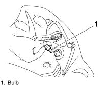
4. Insert a new bulb into the socket.
