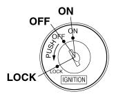
The main switch/steering lock controls the ignition and lighting systems, and is used to lock the steering. The various positions are described below.
