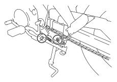
The operation of the centerstand and sidestand should be checked before each ride, and the pivots and metal-tometal contact surfaces should be lubricated if necessary.
