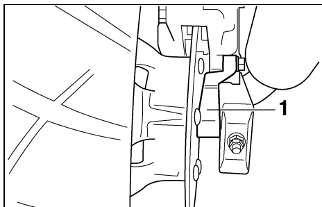
1. Caliper bracket
