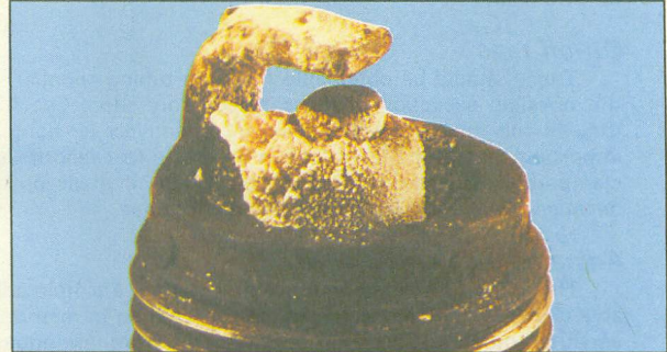
Ash deposits – Light brown deposits encrusted on the electrodes and insulator, leading to misfire and hesitation. Caused by excessive amounts of oil in the combustion chamber or poor quality fuel/oil
