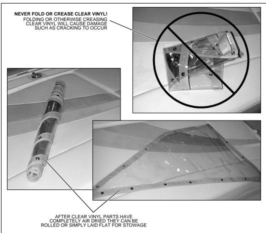
Regularly clean the clear vinyl to prevent dirt, pollen, and etc. from marring the surface. Generally, it is easiest to clean the clear vinyl while it is installed on the boat.
