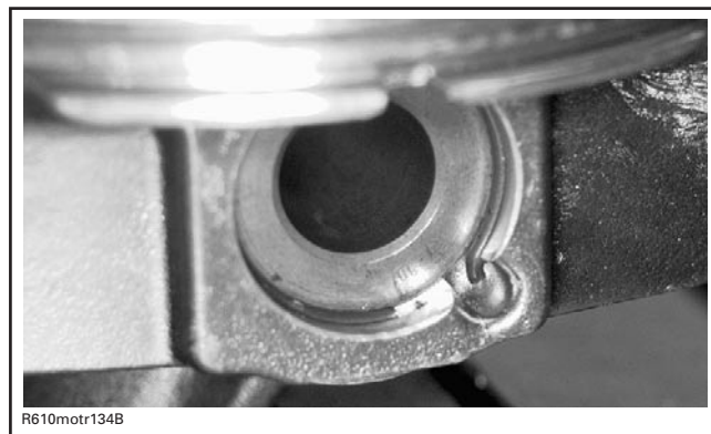
CORRECT POSITION OF THE PISTON CIRCLIP
