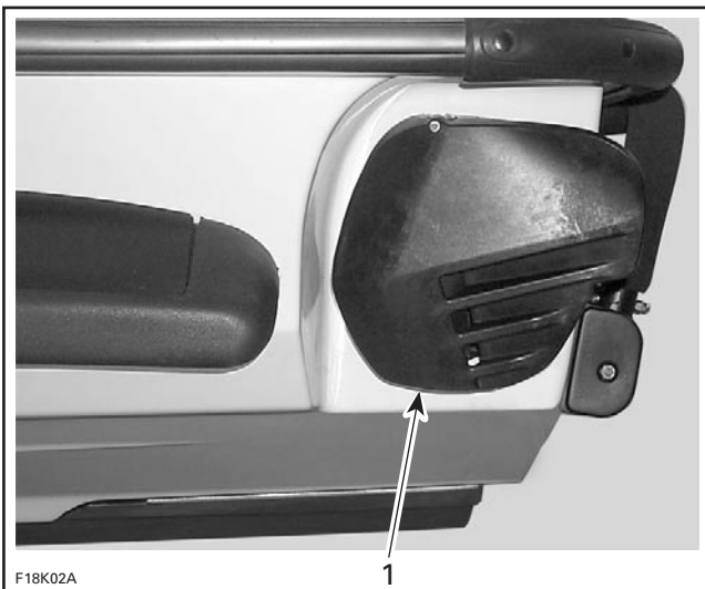
1. Side vane in upper position
