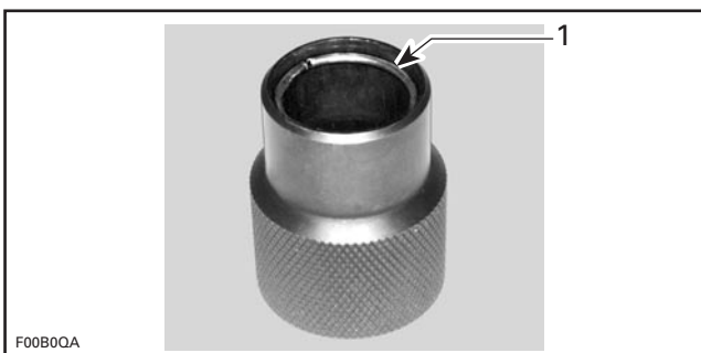
1. Circlip near end of tool
