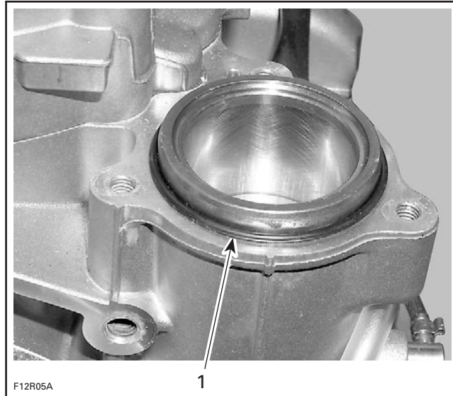
1. O-ring on top of cylinder sleeve
