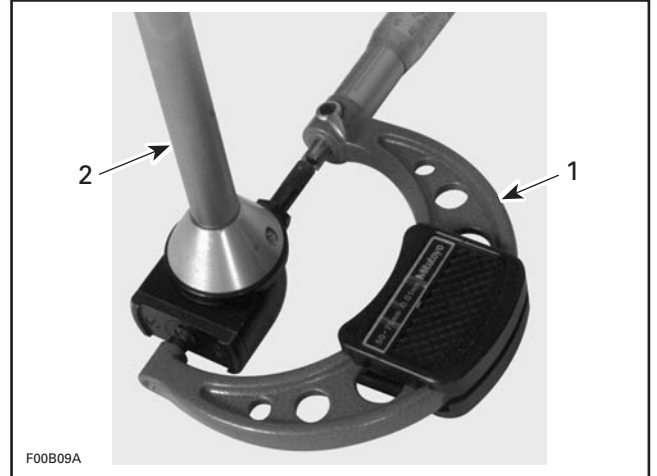
1. Use the micrometer to set the cylinder bore gauge 2. Dial bore gauge
