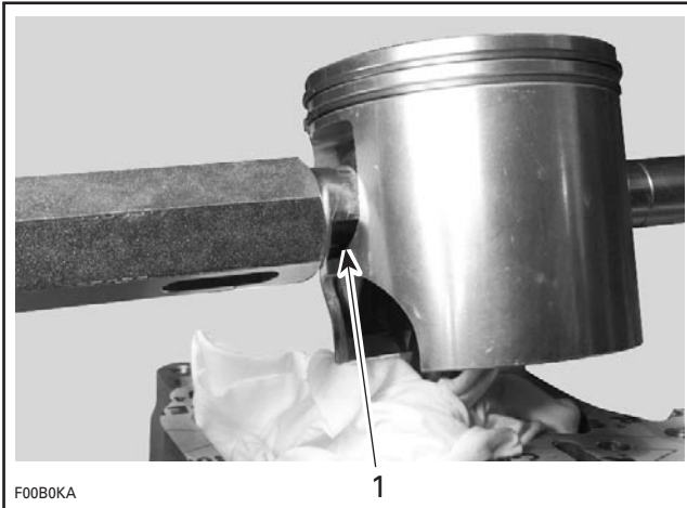
1. Tool cut-out toward bottom of piston
