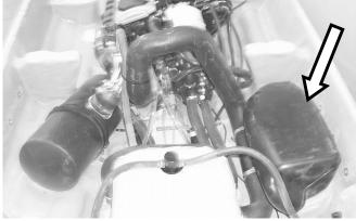
The exhaust junction with the hull is now assembled with silicone and a gasket
