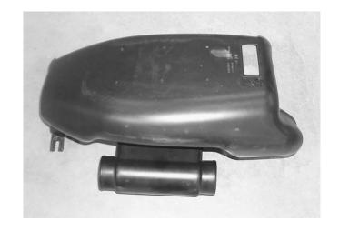
The inside material of the exhaust goose neck is specific to the 4-TEC Intercooled Supercharged. It is calibrated to endure the higher operating temperatures.
