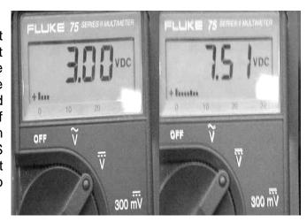
In order to measure the voltage as described above, the 2 pin connector must be connected to the blow-by soleniod, and probed from the backside of it. If the connector is probed from the front side of it when it's disconnected, battery voltage will be read. The low voltage requires less amps and allows the solenoid to run cooler.
