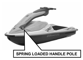
The handlebars are adjustable in 3 different positions to maximize the rider's comfort in all 3 "experiences" of the 3D. Simply press the lever located in the center, under the handlebars.
