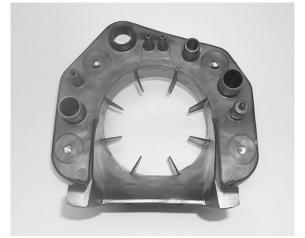
Fins are part of the new design, to help maintaining stable RPM when steering left or right.
