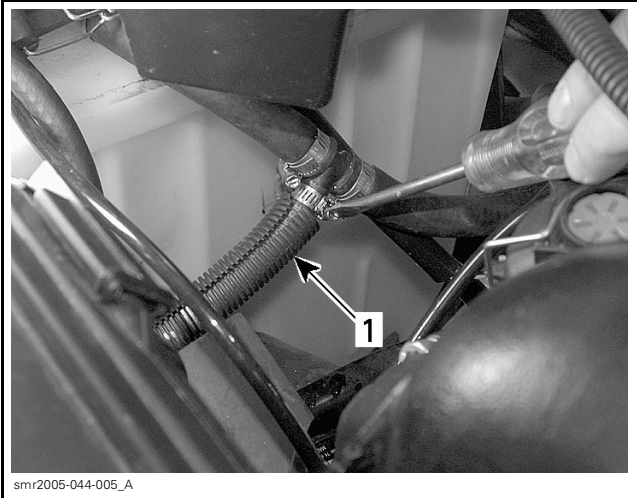
1. Tuned pipe water supply hose
