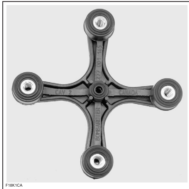
GASKET INSTALLED ON SUPPORT PLATE
