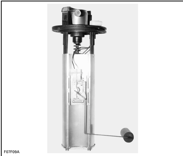
TYPICAL — FUEL LEVEL GAUGE SENDER MOUNTED ON FUEL PUMP MODULE
