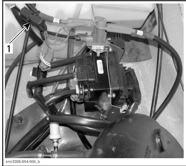
1. Fuse holders of the main fuse (VCM and charging fuse)
