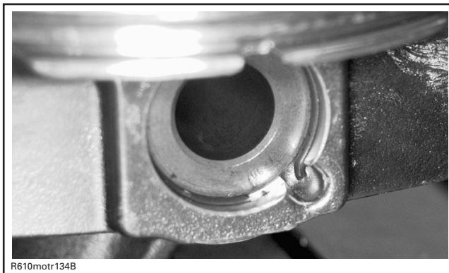
CORRECT POSITION OF THE PISTON CIRCLIP
