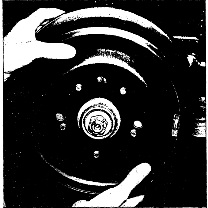
Fig. 18—Aligning Drum Tang with Wheel Hub
