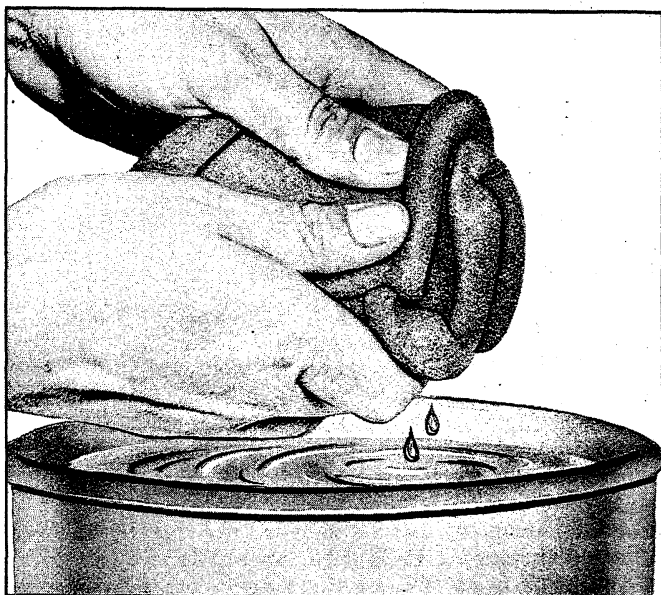
Fig. 3A—Cleaning Polyurethane Element
