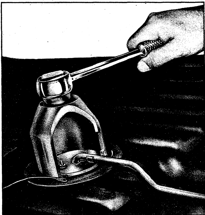
Fig. 5—Meter Assembly Removal Using Tool J-22554
