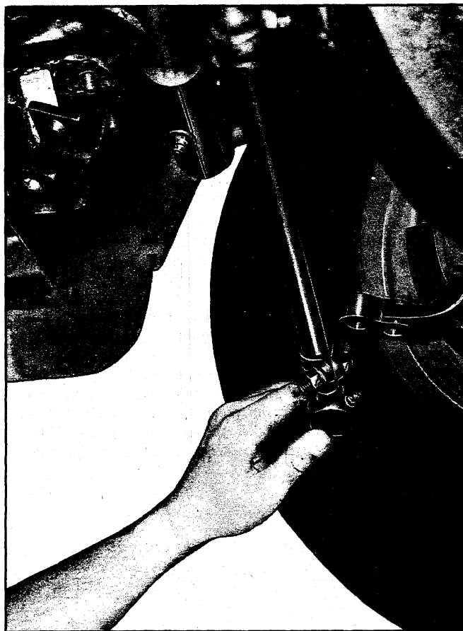
Fig. 6—Adjusting Steering Ratio—Corvette
