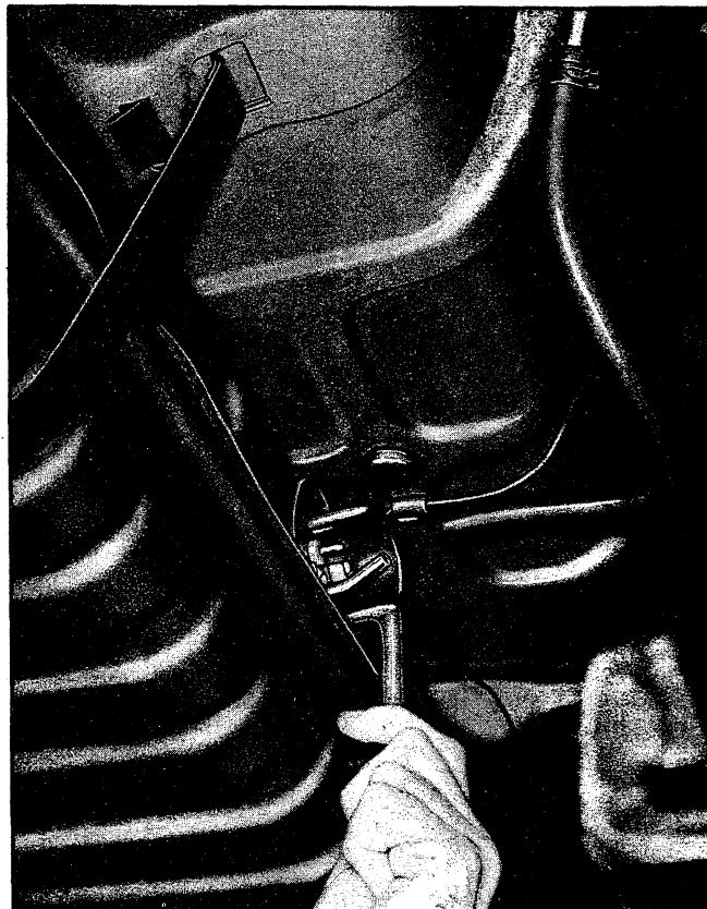
Fig. 12—Fuel Tank Gauge Unit Removal
