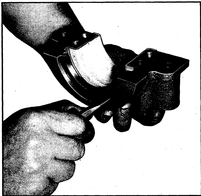
Fig. 10V - Removing Oil Seal (Lower Half)
