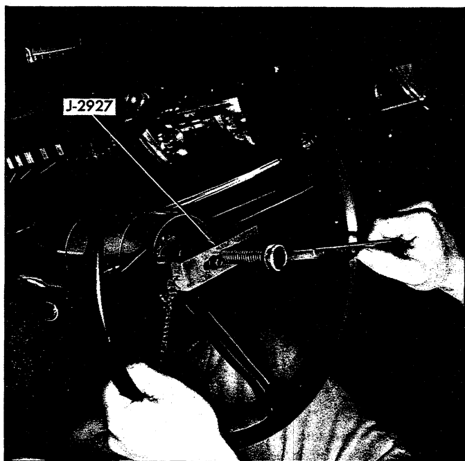
Fig. 9—Removing Steering Wheel with J-2927
