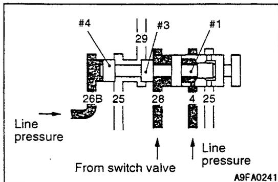
**(4) Fail-safe (when the control relay is off)**
