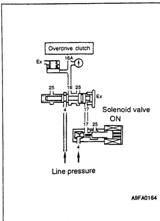
**Pressure control valve and solenoid valve**
