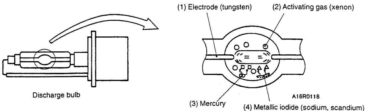
1. By applying a high voltage between the (1) electrodes, the (2) activating gas (xenon) discharges as sparks.
