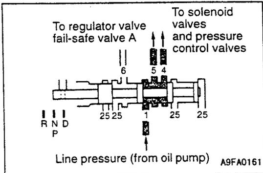
(2) When the manual valve is in the D range position, the No.4 and No.5 ports are opened, and in addition to the valves mentioned in (1), line pressure is also applied to the solenoid valves and pressure control valves for the 2nd brake, underdrive clutch, overdrive clutch, damper clutch and fail-safe valve C.
