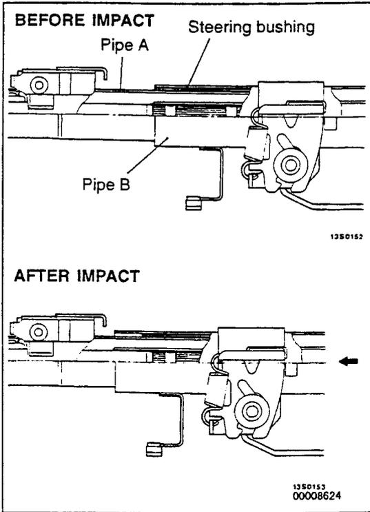
(2) When the pipe B slides forward, the ball inside the steering column bushing absorbs the shock by rolling resistance between pipes A and B.
