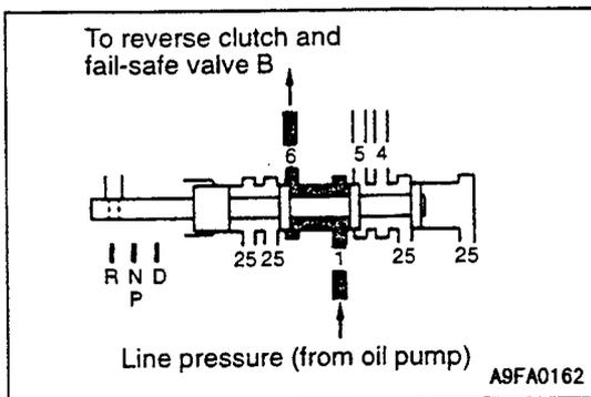
(3) When the manual valve is in the R range position, the No.6 port is opened and the line pressure is applied to the reverse clutch and to fail-safe valve B.
