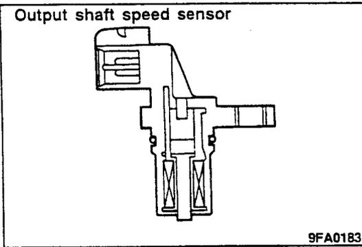
**Input shaft speed sensor and output shaft speed sensor**
