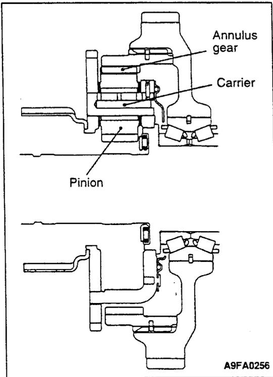
**Direct planetary gear**
