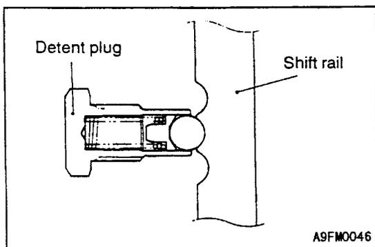
**GEAR DISENGAGEMENT PREVENTING MECHANISM**
