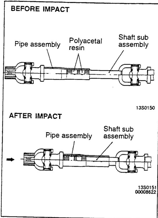
**Shock Absorbing Mechanism**
