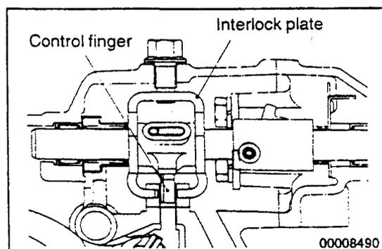
**DOUBLE MESH PREVENTING MECHANISM**
