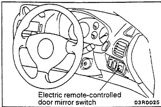
Electric remote-controlled door mirror switch
