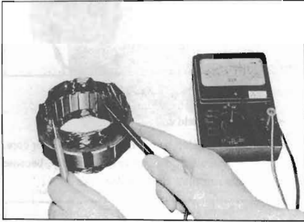
Fig. EE-50 Conduction test
