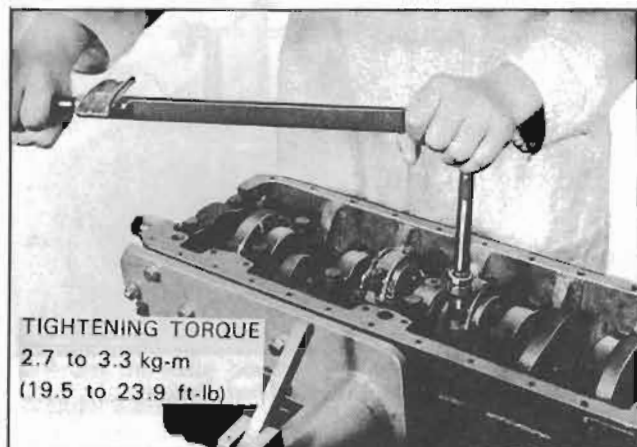
Fig. EM-80 Connecting rod cap installation
