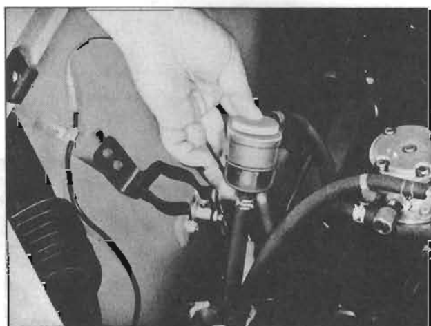
Fig. EF-5 Cartridge type fuel strainer
