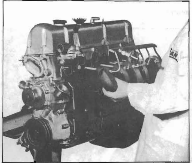
Fig. EM-16 Exhaust manifold removal
