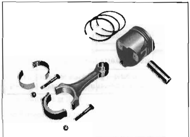
Fig. EM-52 Piston and connecting rod assembly
