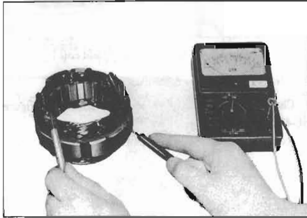
Fig. EE-51 Ground test
