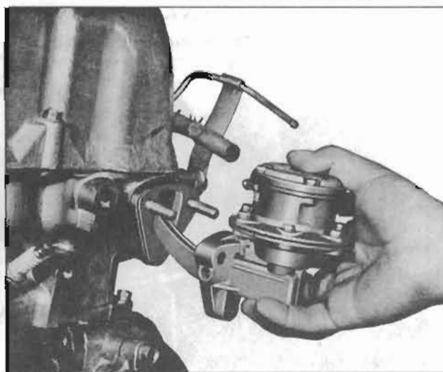
Fig. EM-13 Fuel pump removal
