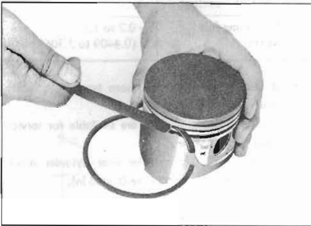
Fig. EM-53 Side clearance measurement
