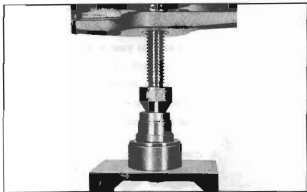
Fig. EC-11 Removing rear rotor bearing
