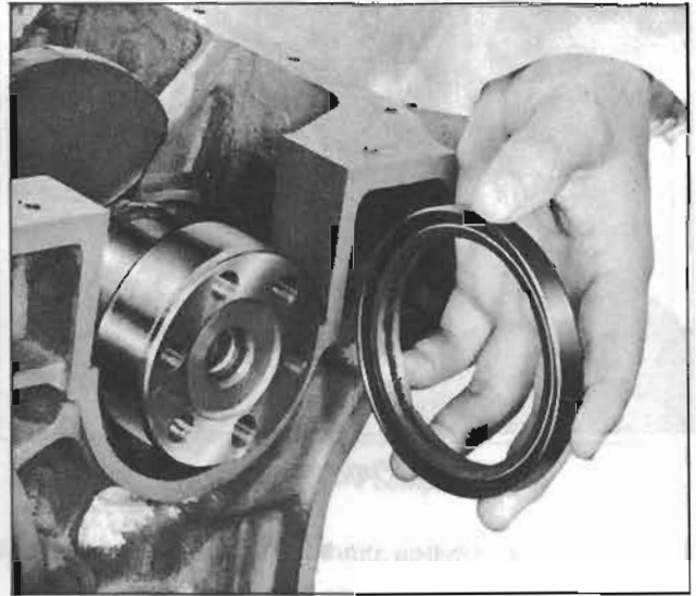
Fig. EM-24 Rear oil seal removal
