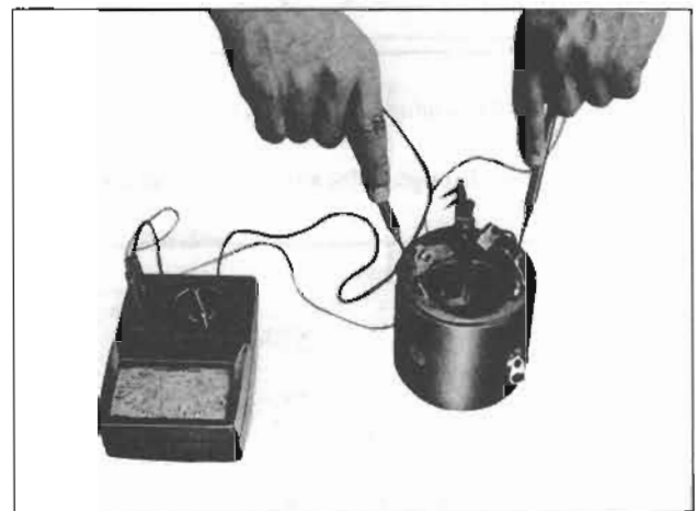
Fig. EE-12 Field coil test for continuity
