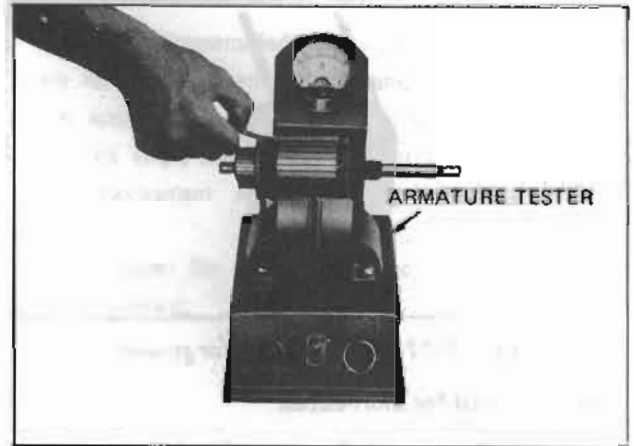
Fig. EE-19 Armature test for shaft
