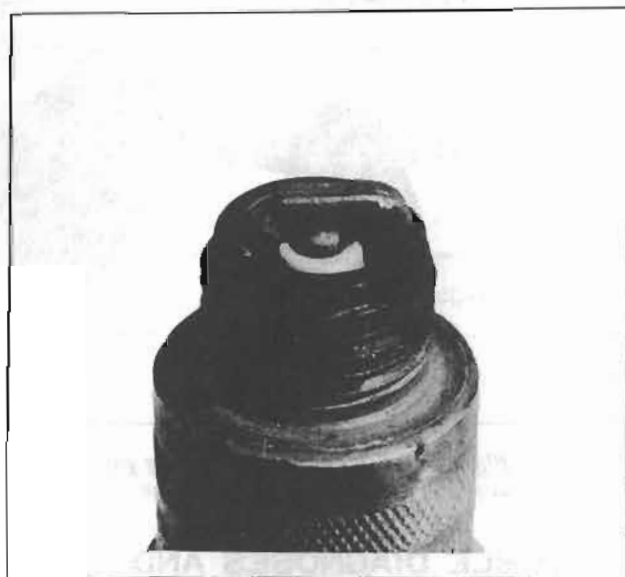
Fig. EE-99 Overheating (III)
