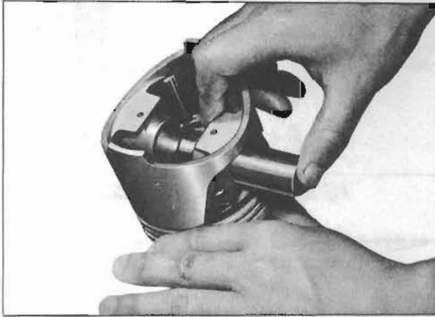
Fig. EM-55 Piston pin fitting
