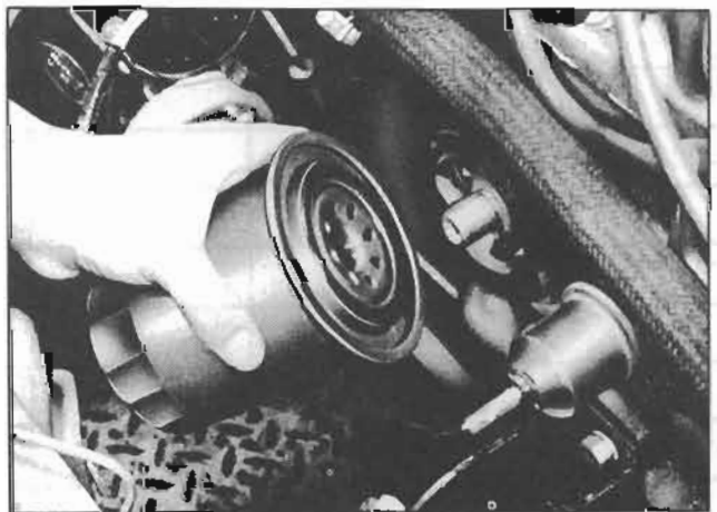
Fig. EL-6 Oil filter
