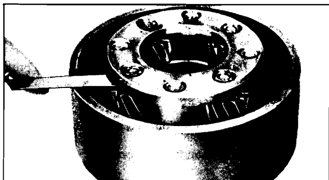
Fig. 7E-117 Checking Reaction Carrier Pinion End Play
