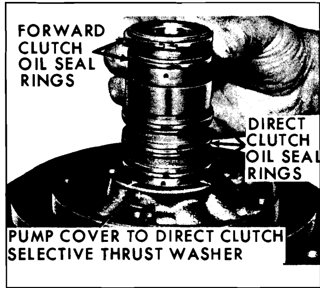
Fig. 7G-48 Removing Oil Seal Rings and Selective Thrust Washer
