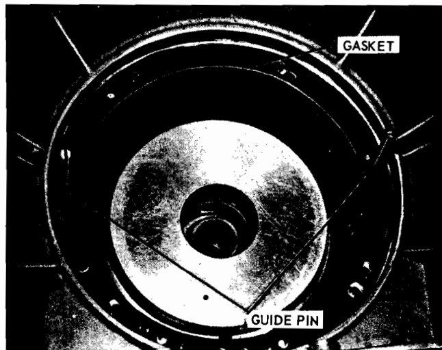
Fig. 7F-106 Guide Pins and Gasket Installed
