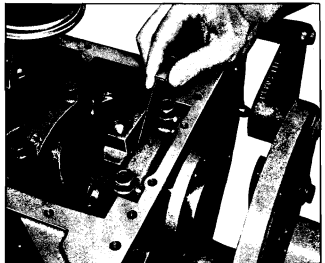
Fig. 6-52 Checking Crankshaft End Play
