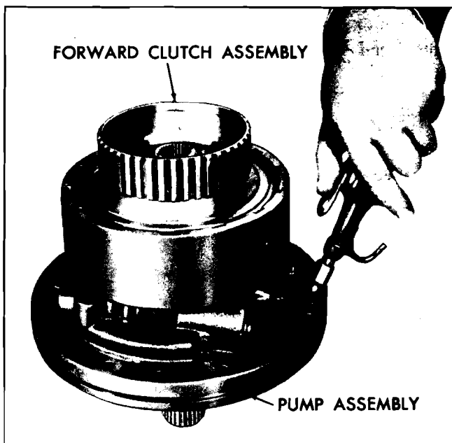
Fig. 7E-92 Air Checking Forward Clutch
