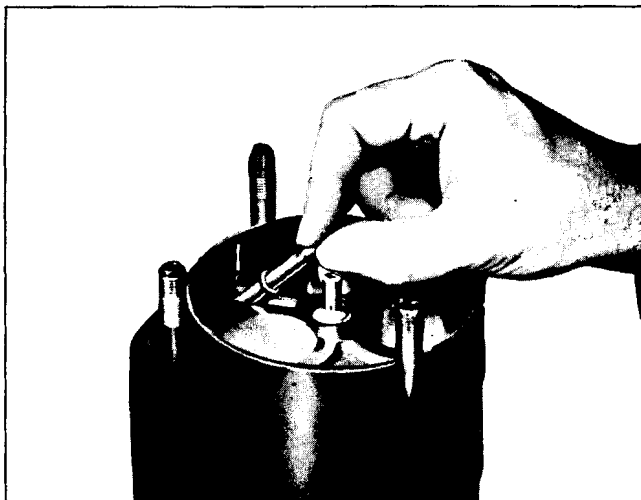
Fig. 1A-42 Installing Oil Intake (Pick-Up) Tube
