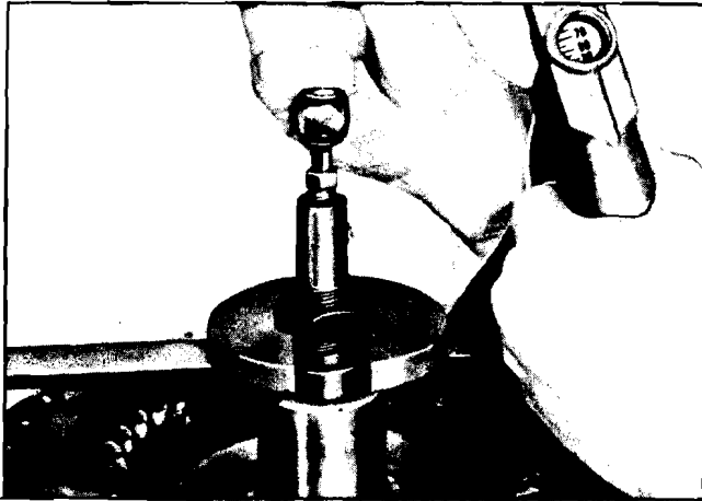
Fig. 7E-132 Air Checking Converter
