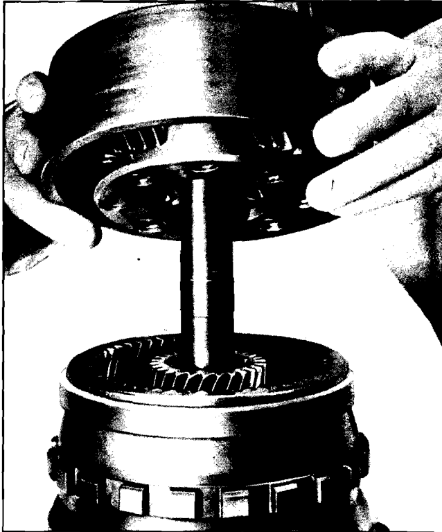
Fig. 7E-142 Installing Reaction Carrier
