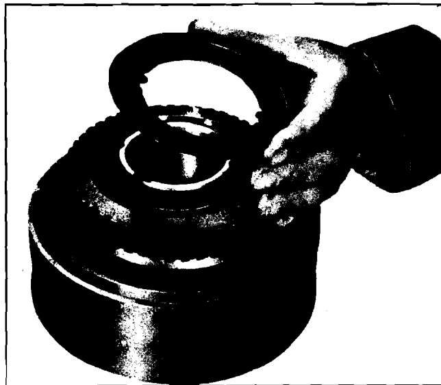
Fig. 7E-109 Installing Intermediate Clutch Retainer
