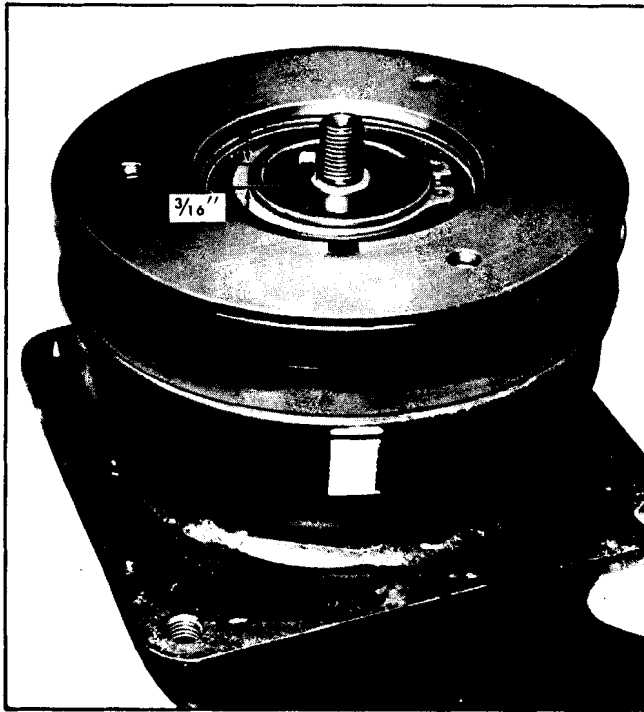
Fig. 1A-7 Proper Position of Hub and Drive Key
