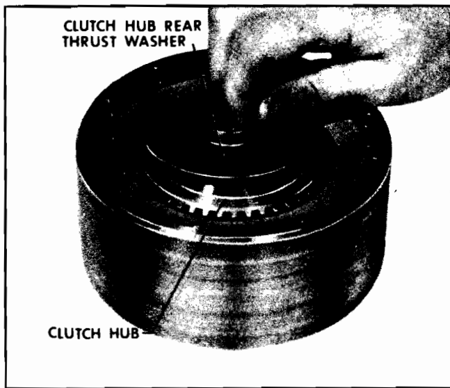
Fig. 7F-48 Removing Clutch Hub Rear Thrust Washer
