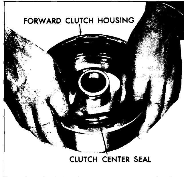
Fig. 7E-86 Removing and Installing Forward Clutch Center Seal
