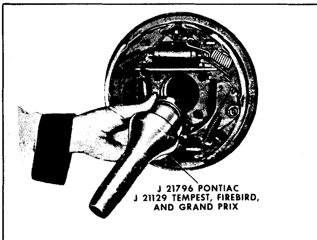
Fig. 4A-14 Installing Axle Shaft Seal (Typical)
