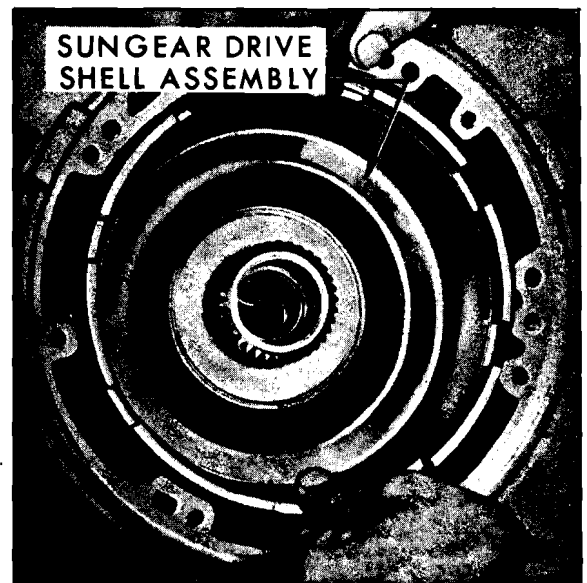
Fig. 7G-29 Removing Sun Gear Drive Shell Assembly
