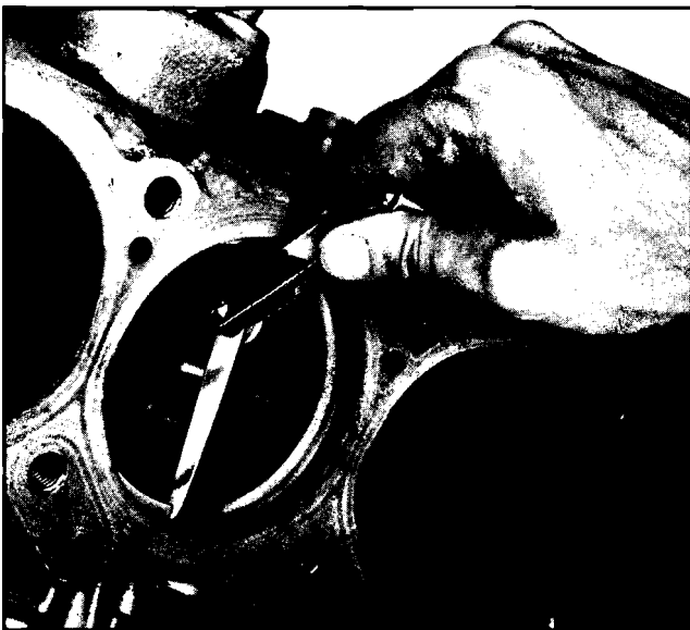
Fig. 6-62 Checking Ring Gap
