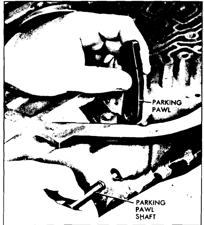
Fig. 7E-39 Removing Parking Pawl and Shaft with O Ring
