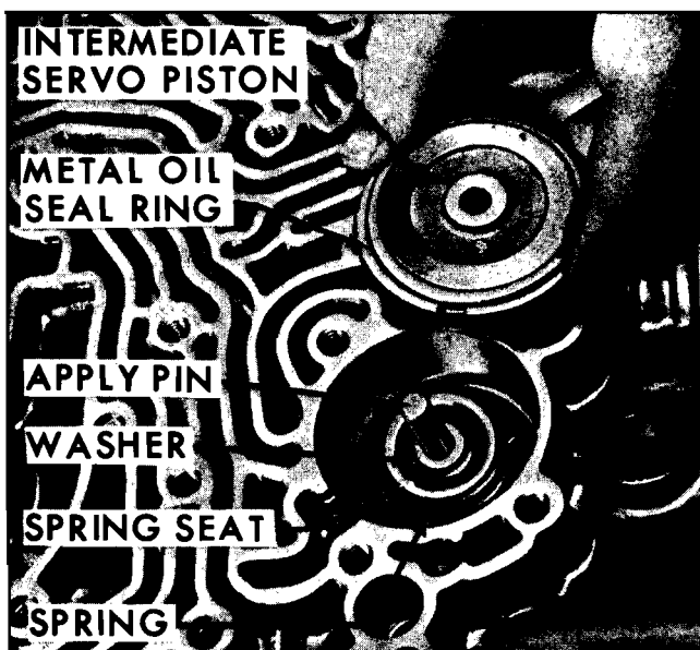
Fig. 7G-23 Intermediate Servo Piston Assembly
