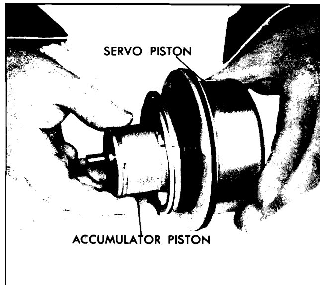
Fig. 7E-64. Removing Rear Accumulator Piston from Rear Servo
