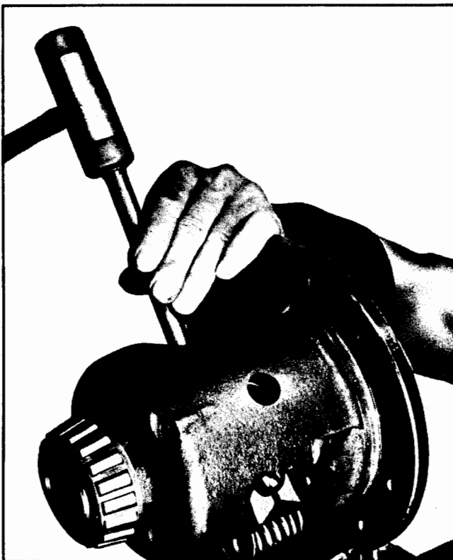
Fig. 4B-5 Removing Preload Springs and Retainer Pontiac
