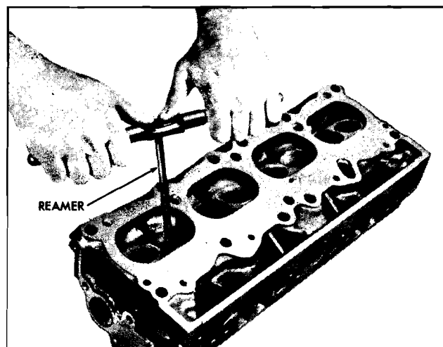
Fig. 6-93 Reaming Valve Guide
