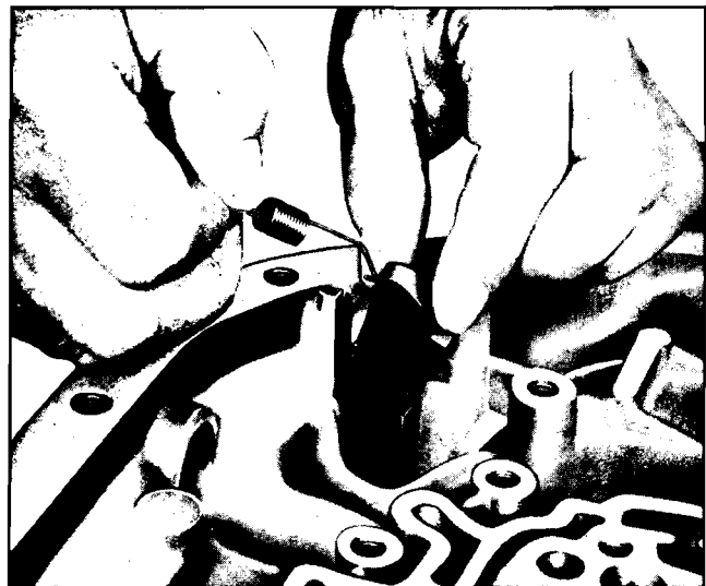
Fig. 7E-36 Removing Parking Pawl Return Spring
