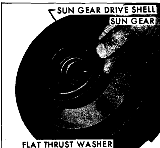
Fig. 7G-85 Removing Rear Flat Thrust Washer
