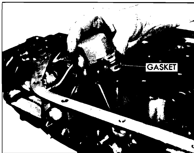
Fig. 7E-22 Removing Detent Solenoid and Gasket
