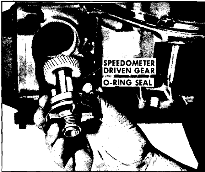
Fig 7E-181 Installing Speedometer Drive Gear and Sleeve
