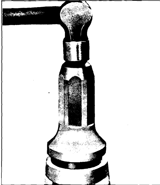
Fig. 7E-166 Installing Rear Extension Seal
