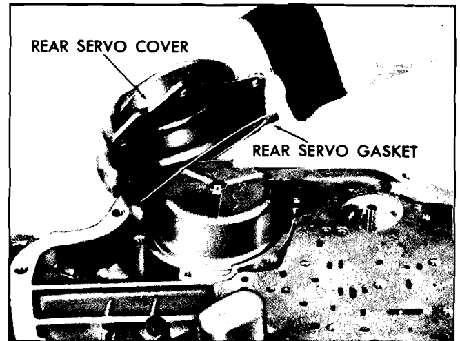
Fig. 7E-175 Installing Rear Servo Cover and Gasket
