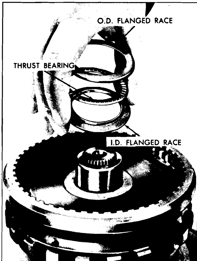
Fig. 7E-139 Installing Rear Internal Gear to Output Shaft Bearing and Races
