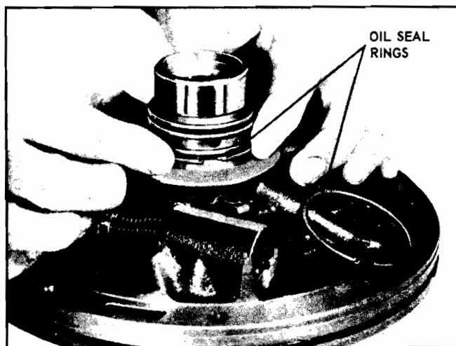
Fig. 7F-111 Installing Oil Seal Rings
