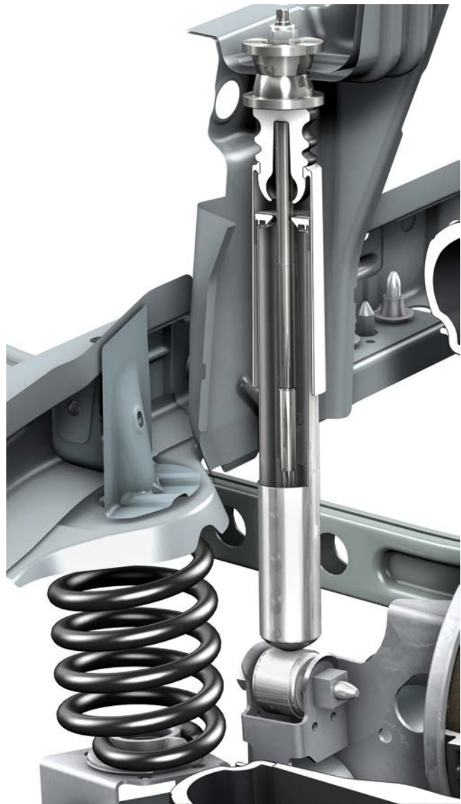
Sectional view of rear axle damping/springing
