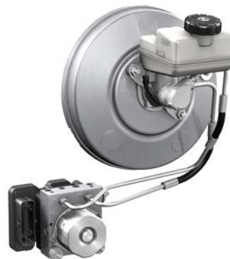
View of brake control system
