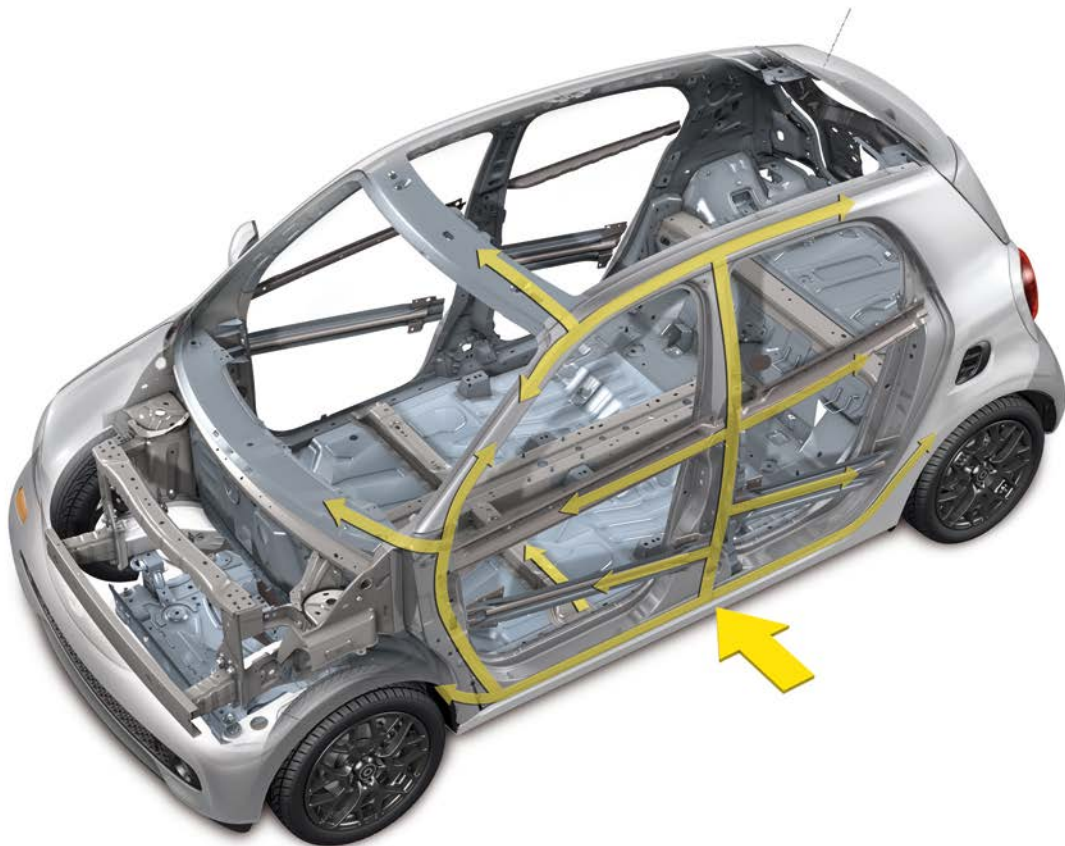
Main load paths in bodyshell during side impact W453
