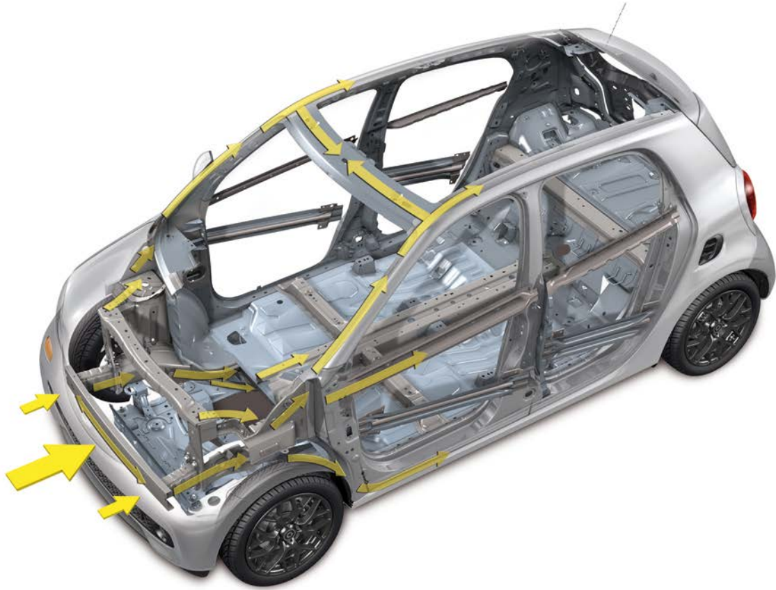
Main load paths in bodyshell during head-on collision W453
