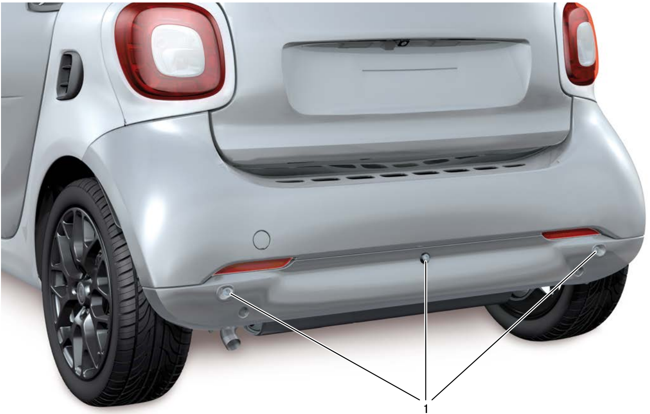
Location of ultrasonic sensors in bumper
