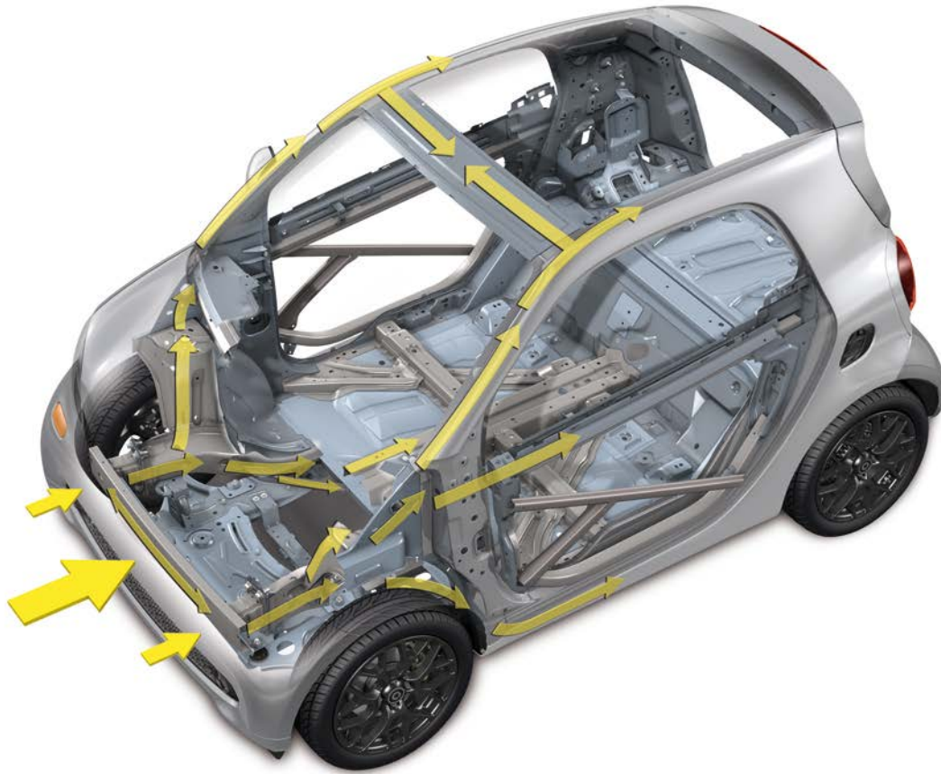
Main load paths in bodyshell during head-on collision C453
