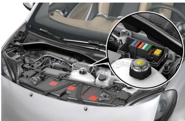
Front compartment fuse box
