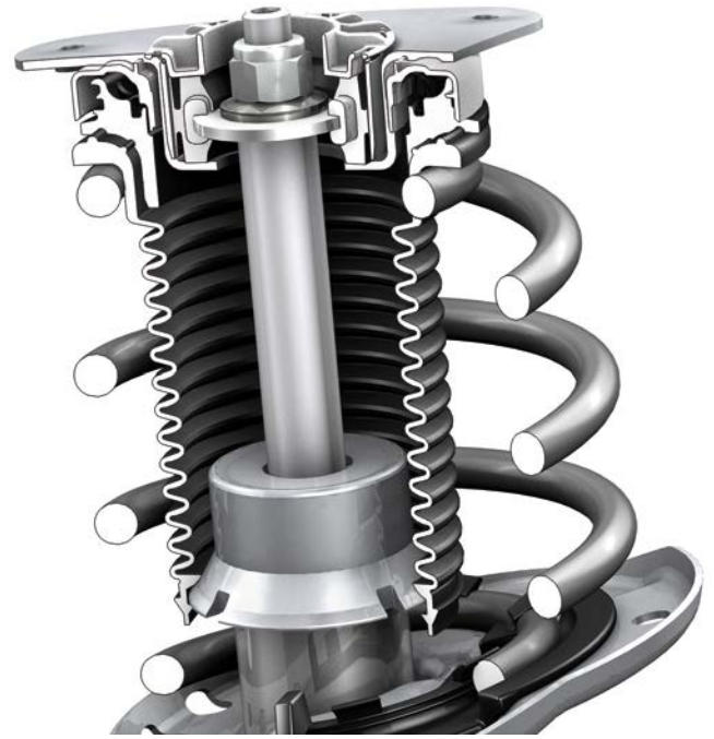
View of support bushing
