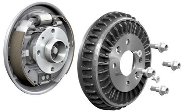
View of rear brake system
