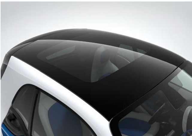
View of panoramic roof incl. sun protection on C453
