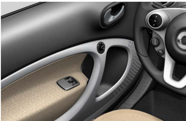
View of power window switch group, driver side
