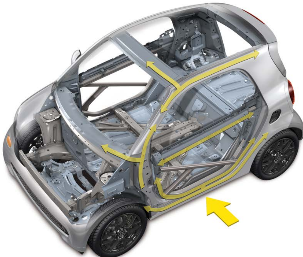
Main load paths in bodyshell during side impact C453
