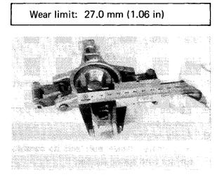
5. Inspect the slides in the sliding sheave for scratches or other damage; replace the sliding sheave as required.
