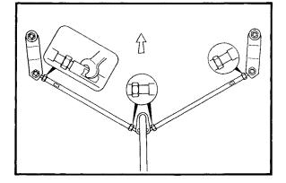
2. The height of the handlebars can be adjusted to suit the rider's preference. After adjusting the handlebars, alternately tighten the four securing bolts. Maintain the specified gap in the steering clamps. Torque the bolts to specification.
