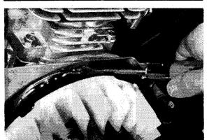
10. Remove the dial gauge stands. Reinstall the starter and the spark plug. Torque the plug to specification.
