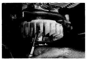
9. Rotate the coil plate by using a screwdriver at the pry points. Align the marks on the coil plate with the mark on the flywheel. Tighten the screws and torque them to spec.
