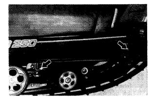
Tightening torque: 4.5 m-kg (33 ft-lb)
