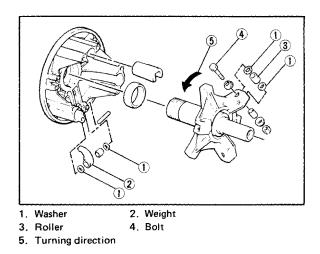
5. Install the primary sheave cap onto the spider as shown.
