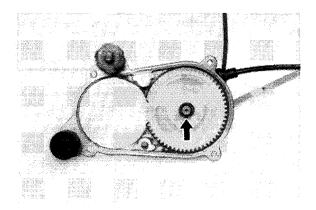
6. Grease the edges of the drive gear, and install the gear case cover.
