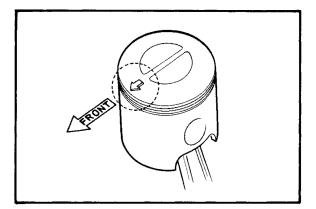
6. Oil the piston pin, and install it in the piston. Be sure the piston pin clip is correctly seated in the groove.
