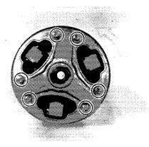
2. Remove the sliders, rollers and weights.
