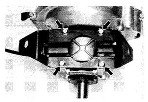
2. Remove the four crankcase bolts. Note the position of the wire bracket. You will have to reinstall it on the same bolt.
