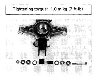
7. Disassemble and inspect the spider levers; replace any worn parts. Reassemble the levers with new cotter pins.
