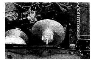
6. Install the key in the jackshaft, and install the fixed sheave. Grease the indicated point.
