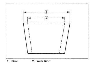
3. Measure the length of the V-belt. It should be within specification; if not, replace the belt.
