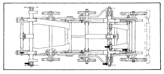
Thoroughly grease the axle in the front pivot arm. Tape the end caps in place. This will hold the axle within the pivot arm during installation of the suspension.
