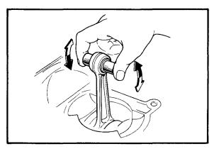
e. The piston pin should have no noticeable free play in the piston. If the piston pin is loose, replace the pin and/or piston.
