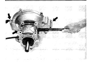
5. Install the engine bracket onto the crankcase. Torque the four bolts to specification.
