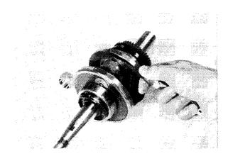
c. Check the crankshaft assembly runout with a dial gauge. If the runout is not within specification, the crankshaft parts are not properly aligned. To correct this misalignment, tap the flywheel with a brass hammer. Use a wedge if necessary.
