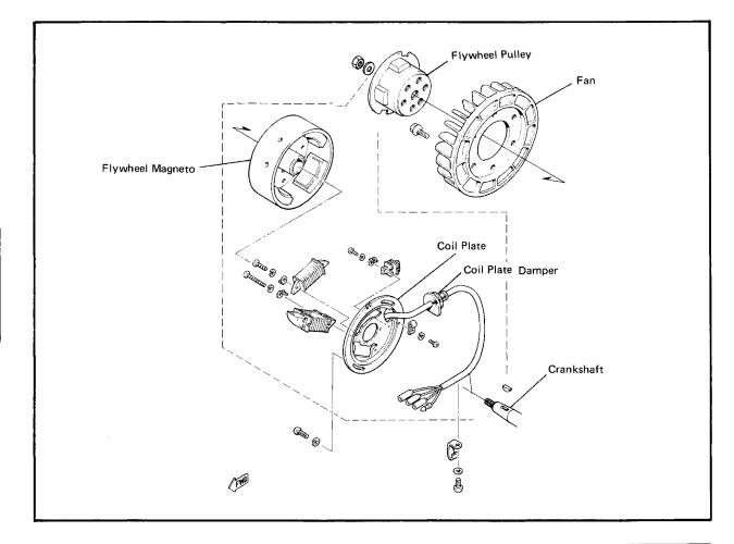
Using the rotor holding tool, loosen the securing nut, and remove the flywheel pulley from the magneto.
