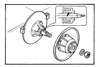
7. Install the washer and securing nut. Torque the nut to specification.
