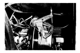
3. Remove the clevis pin and disassemble the brake.
