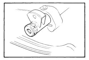
Place the suspension in the track, and swing it into place in the chassis. Install both front suspension-mounting bolts. Do not tighten them at this point.
