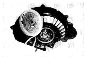
Install the drive pawl and the return spring. Hook the spring around the first post on the sheave drum as shown in the photograph.
