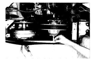
If either the center-to-center distance or the offset is not within specification, check the engine mounts. If the engine has been mounted correctly, the engine mounting bracket, the frame, or both are bent. Replace as required.
