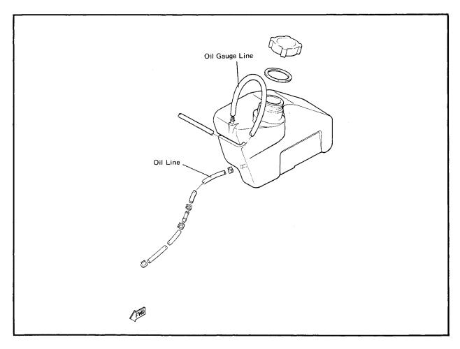
1. Check the oil line from the tank to the pump. It should be free from all obstructions and should not be pinched or
