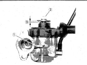
1. Oil pump gear 2. Plunger 3. Minimum pump stroke
