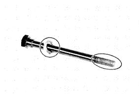
3. Tighten the mounting bolts with the special tools to specification.
