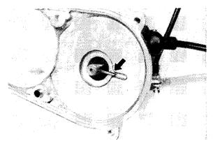
5. Remove the drive shaft from the oil pump. Inspect the bearing surfaces of the shaft and the gear teeth. If any part of the shaft is worn or pitted, the shaft must be replaced.
