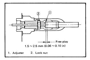
Free play between outer tube end and adjuster:  $1.5 \sim 2.5 \text{ mm} (0.06 \sim 0.10 \text{ in})$
