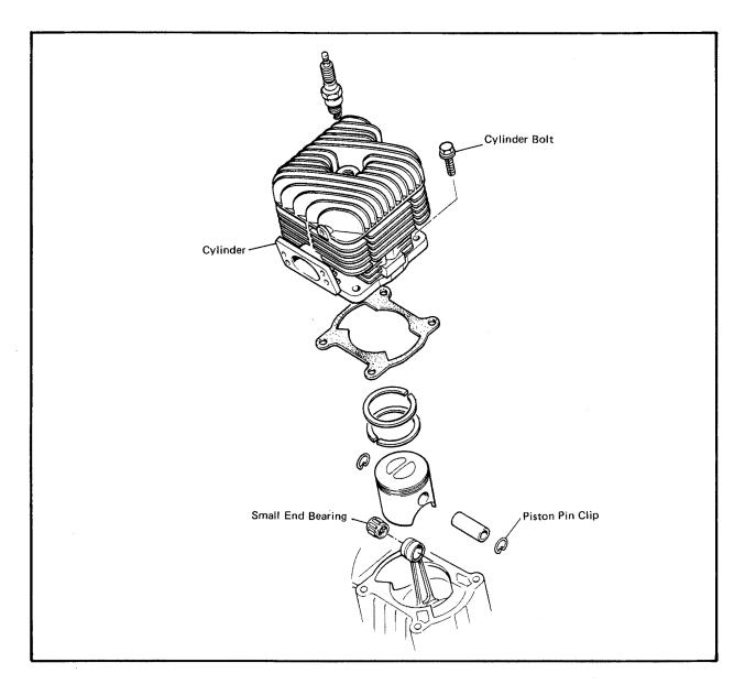
1. Install the piston rings as shown in the illustration.
