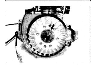
5. Install the flywheel pulley. The two cutouts on the edge of the pulley must be opposite the holes in the fan. Torque the securing nut to specification.
