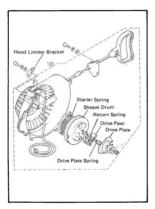
1. Hook the outer book of the starter spring around the post in the starter case. Carefully wind the spring counterclockwise, and fit the spring into the case. Thoroughly grease the spring after installation.
