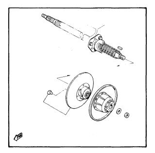
5. Starting from the free position, rotate the sliding sheave clockwise to preload the spring, and push the sheave towards the chain case. Lock the sliding sheave in place with the secondary sheave holder.
