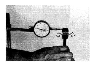
b. Check the connecting rod side clearance at the big end. If it exceeds specification, disassemble the crankshaft and replace any worn parts.
