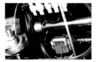
5. Tighten the chain case bolts and torque them to specification.
