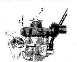
If either the maximum pump stroke or the minimum pump stroke does not equal specification, remove the adjusting plate and add or remove adjusting shims as required. Adding shims increases the stroke, removing shims decreases the stroke.
